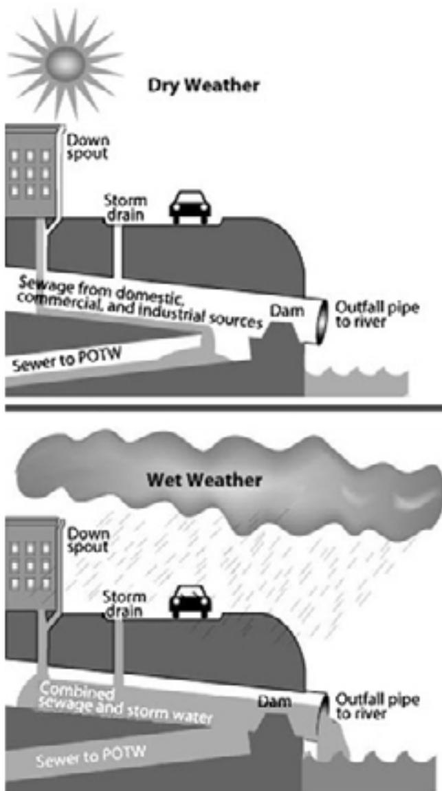
**Figure 2.** Under normal conditions, a combined sewer system distributes all sewage to a treatment plant. Heavy rainfall can cause overflows, sending some untreated sewage into nearby waterways. Credit: EPA.
